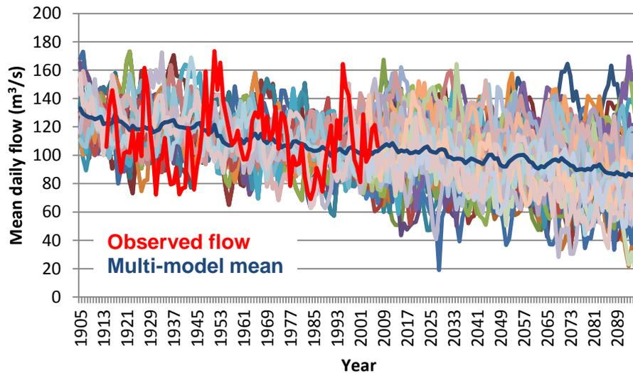
**Figure 1:** Simulated streamflow, for 1905-2096, for the naturalized Oldman River near Lethbridge. Each simulation corresponds to one of 50 runs of ten CMIP3 global climate models. The greenhouse gas forcing is according to the moderate A1B emission scenario. The observed gauge record (red) and all-model mean (dark blue) also are plotted. Daily mean flow smoothed by a 5-point binomial filter.
