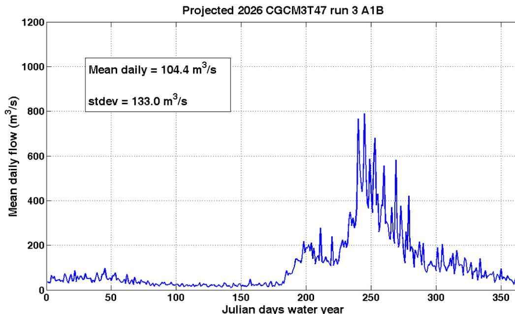
**Figure 8:** Projected mean daily flows for 2026 for the naturalized Oldman River near Lethbridge simulated using output from the GCM CGCM3T47 run 3, GHG emission scenario A1B. Scale same as in Figure 6.
